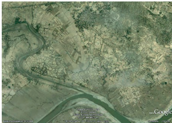
Figure 27 — Active and paleo-channels. During major flood events such paleo-channels are the first to be inundated or even reactivated. Near Indus River, Uttar Pradesh, India, 26°26' N, 79°11' E (Google Earth, accessed March 2013)
